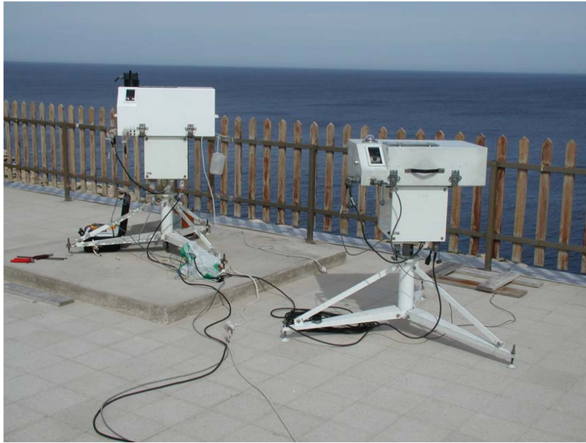
Figure 2.1.1. Picture of the Brewer MKIII #123 (left) and the portable Brewer #017 (right) on the roof of the ENEA Laboratory at the island of Lampedusa.
