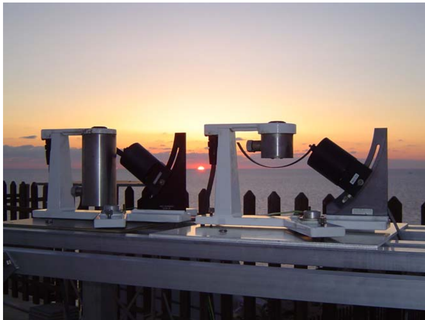
Figure 2.1.4. The Multifilter Rotating Shadowband Radiometer MFR-7 (right side) and UVMFR-4 (left side) at Lampedusa
