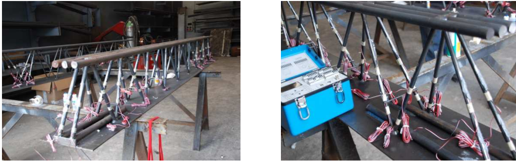
Figure 2. Sample C : strain gauges testing before concrete filling
