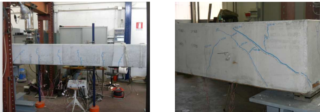
Figure 8. Sample C : cracking pattern
