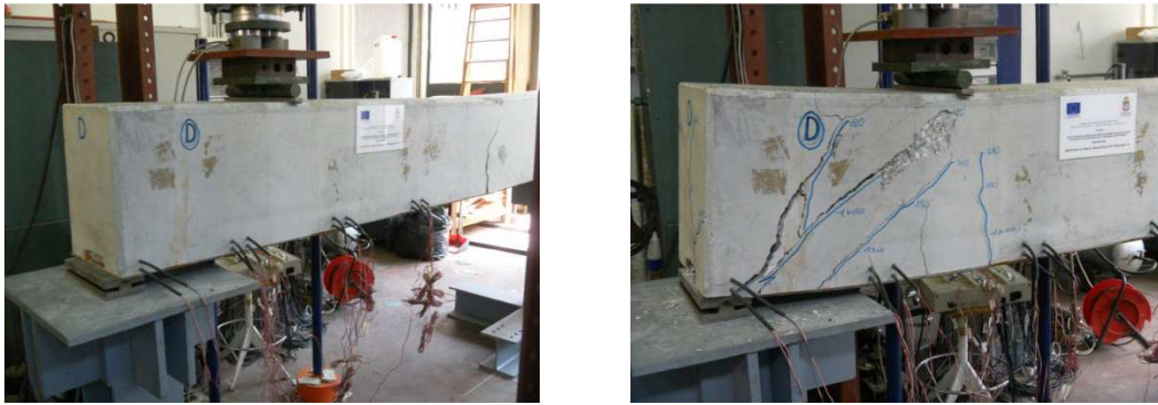
Figure 11. Sample D : cracking pattern
