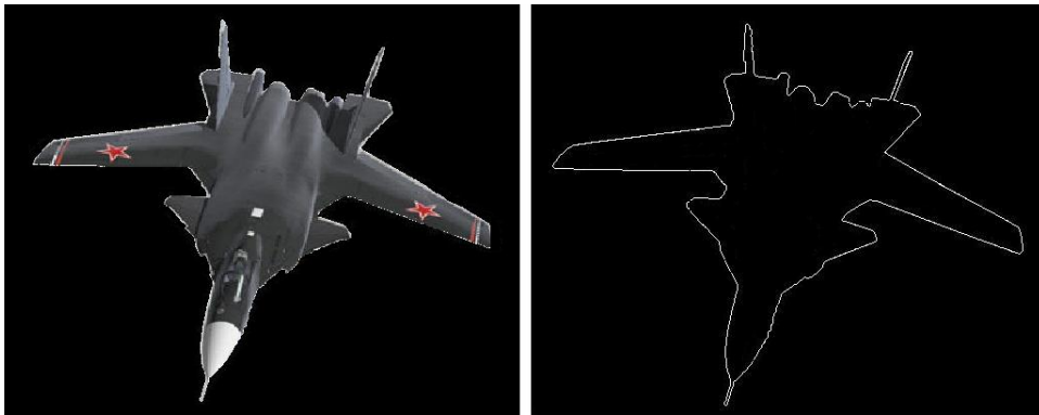
Figure 4.2: An image of an airplane and the contour obtained by using the Canny algorithm.
