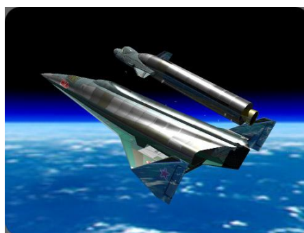
Figure 3 - 11 – Captive on Top concept of the Russian aerospaceplane Spiral
