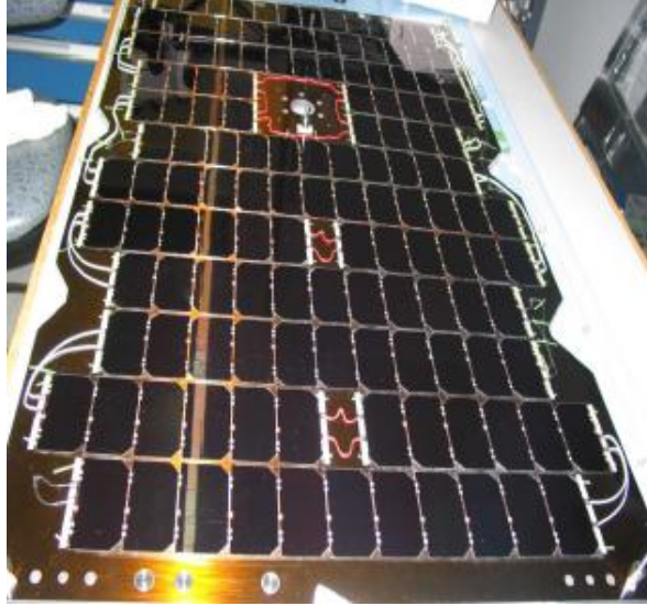
Figure 5 - 40 – Triple junction cells on carbon fibre (CFRP) panel. Courtesy of Surrey SSTL.
