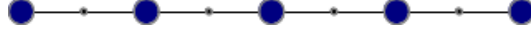
Figure 6.11: Segment made by 5 holes separated by 2. Since N_c = 5 and l_{seg} = 8 , we have \nu = 1/2 .
