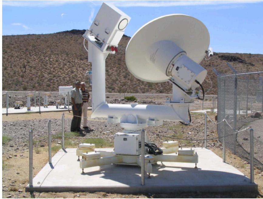
Figure 3.5. Advanced Media Calibration System - Water Vapour Radiometer at DSS-25.
