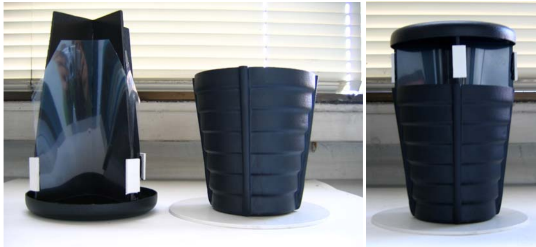
Figure 9 - Photographs showing details of the sticky trap used during mark-release-recapture experiments for collected adult mosquito.
