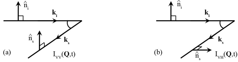
Figure 3.4. Two different pairs of polarization directions used in this work: (a) polarized scattering signal I_{VV} and (b) depolarized scattering signal I_{VH} .
