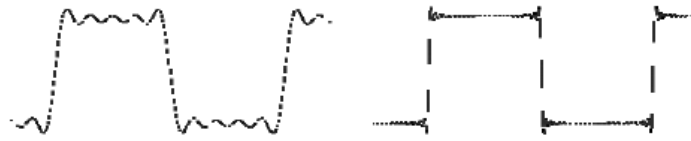
Fig. 1-2: Gibbs effect on a filtered square wave signal [6].
