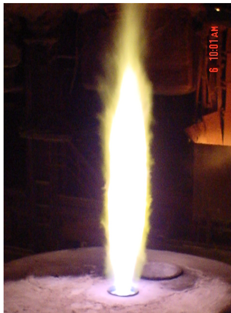
Figure 9.1 Bunsen pipe used to obtain the reactive jet.
