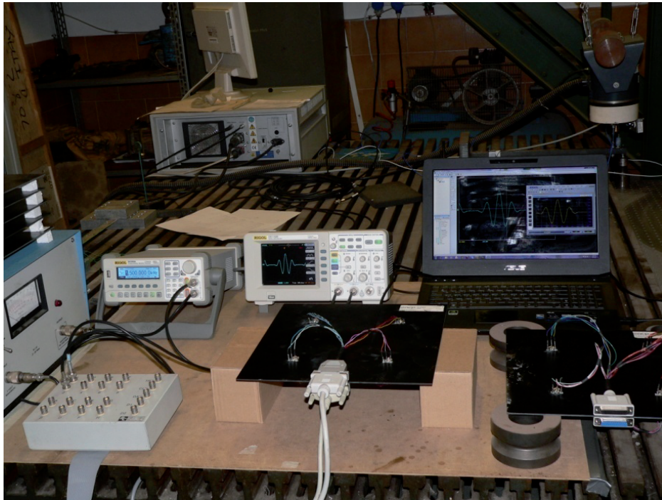
Figure 7.1: The experimental setup for the tests performed to validate the proposed SHM routine.
