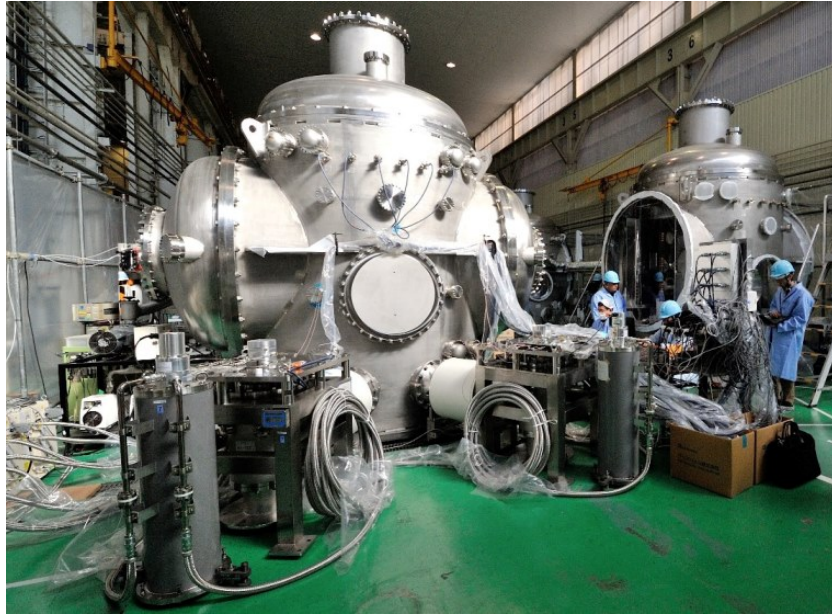
Figure 6.30: Cryostats for the payloads of KAGRA under assembling and testing, at the Toshiba Keihin Product Operations in Yokohama (Japan).
