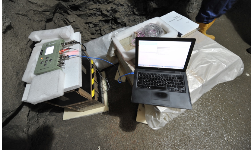
Figure 5.13: The data acquisition system Taurus (on the left), in a temporary setup next to the seismometer Trillium 240 (placed into the external insulation box, on the right side), during the sensor installation.
