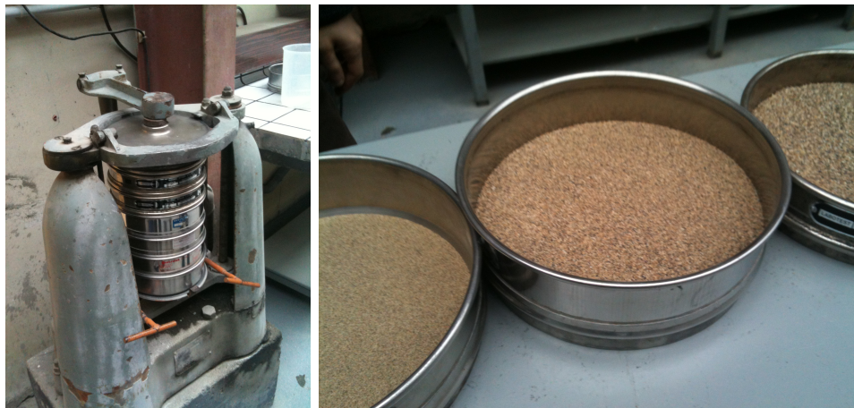
Figure III.2: A sand vibrating sieve machine and some sieve frames.
