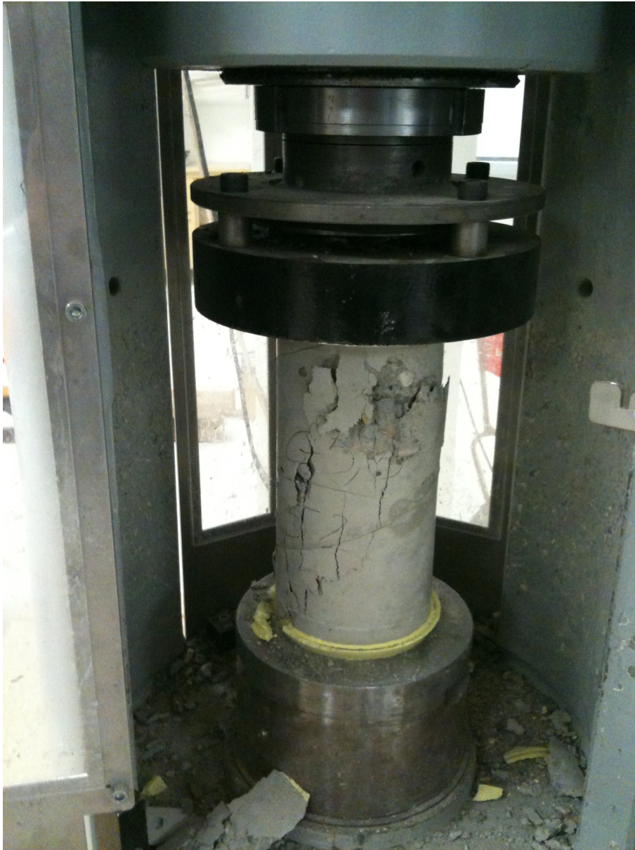
Figure III.6: A ramp test to measure compressive strength.
