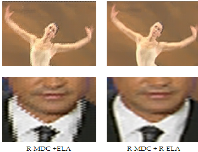
Figure 3.3: Details for frame 46 of the sequences decoded using R-ELA and ELA interpolation, News sequence, CIF, 600 kbps.
