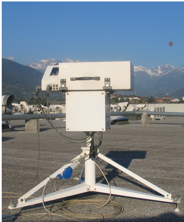
Figure 3.7: Brewer #066 on the terrace of the ARPA Valle d’Aosta building. The main components of the Brewer system may be seen: the spectrometer case (upper part), the tracker (middle) and the tripod.
