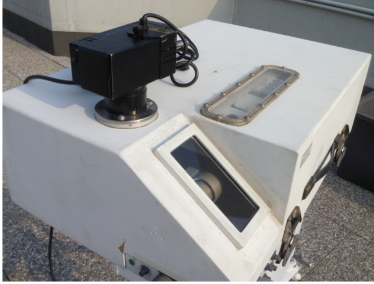
Figure 4.1: One of the lamps used for the dispersion test on Brewer #066. The lamp fits the upper dome normally employed for global UV measurements.
