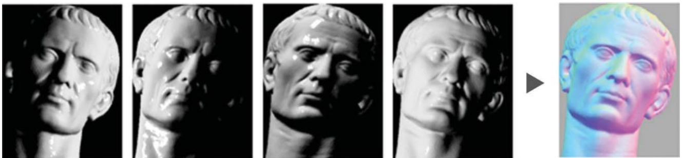
7/ Displacement map obtained from different directions illumination by shape from shading. Machine vision lab, Swiss Federal institute of technology
