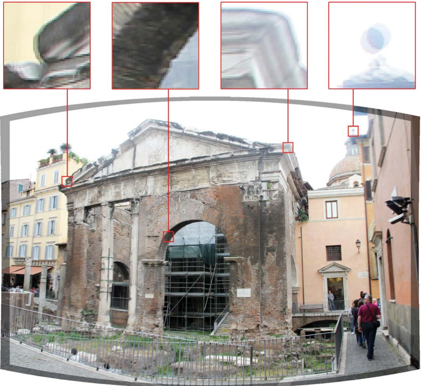
7/ Superimposition of two equirectangular images, the first corrected and projected by PTGui directly and the other corrected using the calibration parameters with other software then just projected with PTGui. The gray frame around is the crop applied to the correct image to have the original image dimensions.
