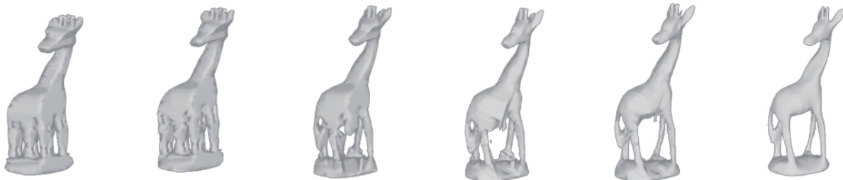
3/ shape from Silhouette model using 2, 3, 4, 6, 9, 20 photos with the software STRATA 3D
