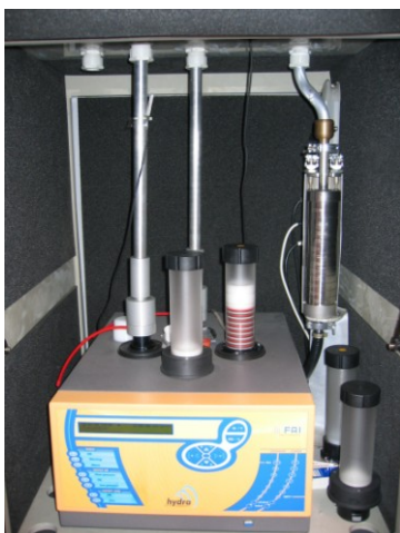
Figure 4.1.3.a.: HYDRA-Dual Sampler and DLPI- Dekati in parallel in the sampling campaign of April, in downtown Rome
