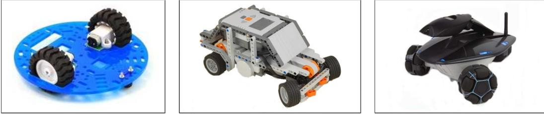
**Figure 1.4** Examples of different wheeled robot types. From left to right: differential drive, car-like and omnidirectional wheeled robot.
