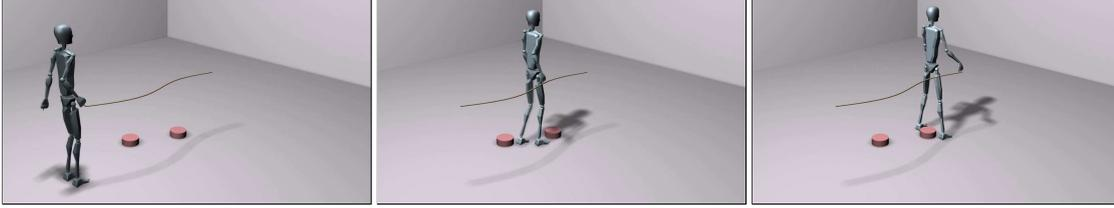
**Figure 4.2** An example of solution for the TCMP problem. (left) The initial state of the robot with the task trajectory assigned for the right hand, aimed for a manipulation task. The motion planner should avoid the obstacles on the ground (red cylinders) while fulfilling the assigned task. (center) An intermediate posture assumed by the robot to fulfil the task and before approaching an obstacle. (right) The final state that completes the assigned task.
