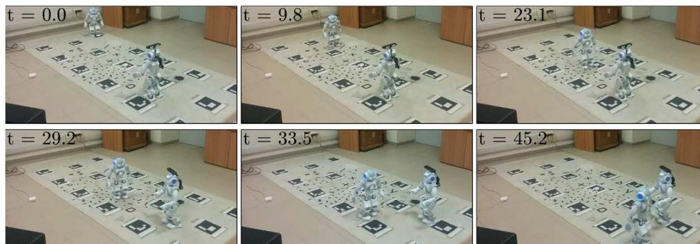
**Figure 7.9** Evasive motion using the *move aside* strategy: snapshots from an experiment.
