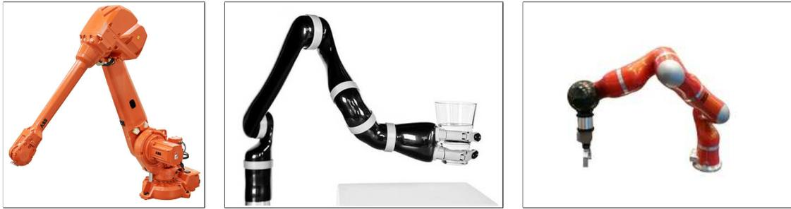
**Figure 1.1** Some examples of manipulator robots. From left to right: an industrial robot from ABB, the KUKA LWR and the KINOVA JACO arm.
