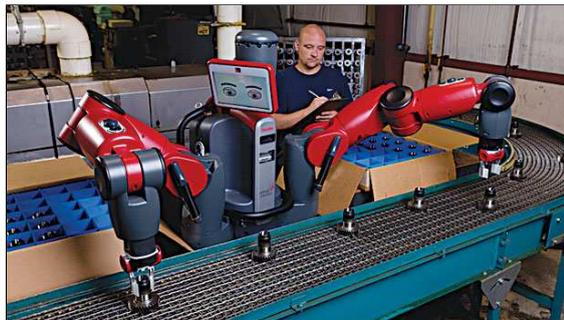
**Figure 2.1** Example of a scenario where the motion planning is fundamental for fulfilling the pick and place task.
