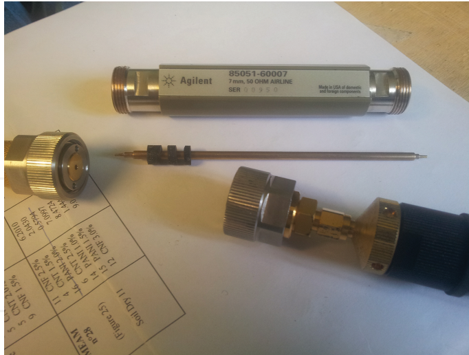
Figure 2. Coaxial airline 50 Ω probe used for the dielectric characterization of nanocomposite materials and for the measurement of EM reflection and transmission properties of layered materials.
