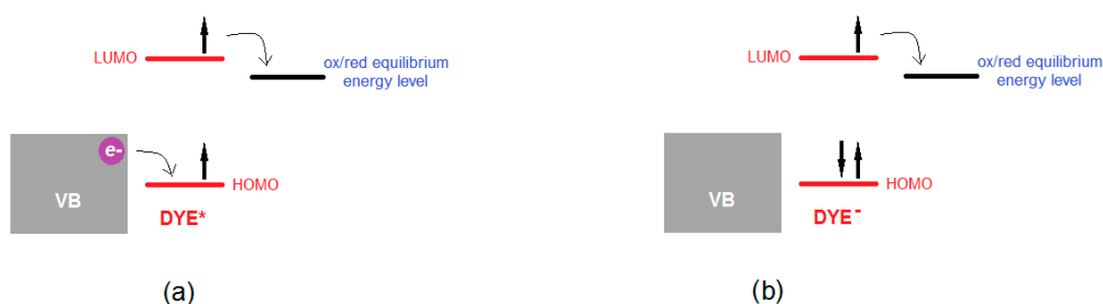
Figure 6. Mechanism of ET between the photoexcited dye sensitizer to the oxidized form of the redox mediator (with the redox energy level (in black) positioned below the LUMO of the dye-sensitizer) in a p -type sensitized cathode of a p -DSC. The relative positioning of the frontier energy levels involved in the photoreduction process is shown. (a): case of ET from the excited dye to the redox shuttle which precedes hole injection in the semiconductor VB (charge injection slower than ET); (b): case of ET from the excited dye to the redox shuttle which follows hole injection in the VB of the semiconductor (ET slower than charge injection). HOMO-LUMO energy separation for the immobilized sensitizer is assumed to be unvaried when the dye passes from the neutral state to (a) the oxidized or (b) the reduced state.
