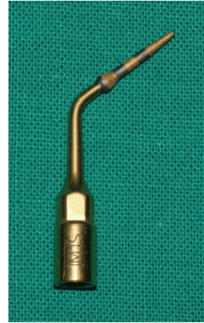
FIGURE 1: The diamond tip (IMIs, Mectron Medical Technology, Carasco, Italy) used in the tests. This tip can be regarded as a pilot drill in piezoelectric implant site preparation.
