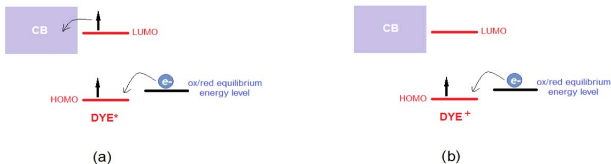
FIGURE 12. MECHANISM AND ENERGY LEVELS INVOLVED IN THE PROCESS OF ELECTRON TRANSFER FROM THE REDUCED FORM OF THE REDOX MEDIATOR TO THE DYE SENSITIZER IN A N -TYPE ANODE OF A T -DSC WHEN: (A) THE ELECTRON IS UPTAKEN BY THE DYE IN THE EXCITED STATE AND PRECEDES ELECTRON INJECTION IN THE SEMICONDUCTOR CB (CASE OF SLOW CHARGE INJECTION); (B) THE ELECTRON IS UPTAKEN BY THE DYE IN THE OXIDIZED STATE AND FOLLOWS ELECTRON INJECTION IN THE SEMICONDUCTOR CB (CASE OF FAST CHARGE INJECTION AND SLOW DYE REGENERATION). THE SEPARATION BETWEEN THE HOMO AND LUMO LEVELS OF THE IMMOBILIZED SENSITIZER IS ASSUMED TO BE THE UNVARIED WHEN THE DYE PASSES FROM THE (A) NEUTRAL TO THE (B) OXIDIZED STATE.
