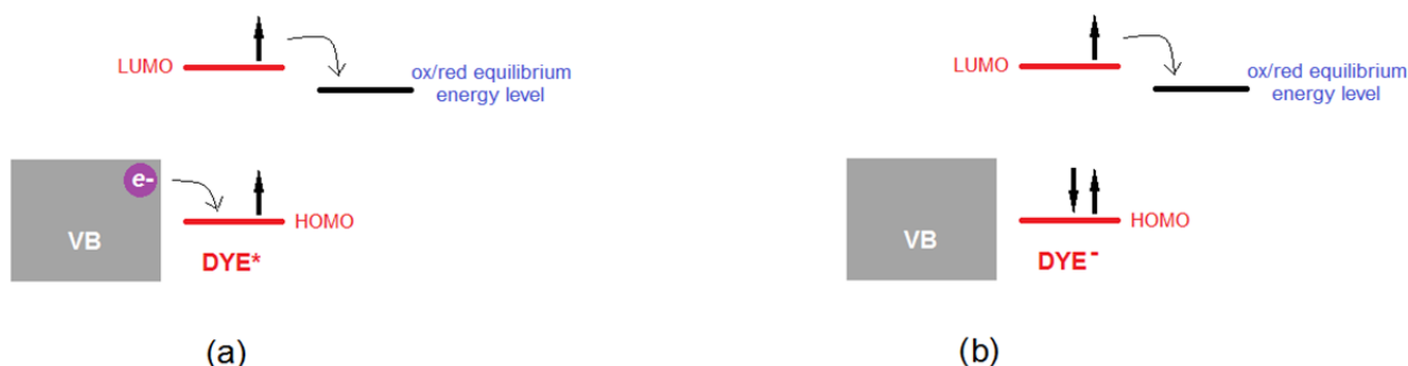
FIGURE 13. MECHANISM AND ENERGY LEVELS INVOLVED IN THE PROCESS OF ELECTRON TRANSFER FROM THE DYE SENSITIZER TO THE OXIDIZED FORM OF THE REDOX MEDIATOR IN A P -TYPE CATHODE OF A T -DSC WHEN: (A) THE ELECTRON IS TRANSFERRED BY THE DYE IN THE EXCITED STATE AND PRECEDES HOLE INJECTION IN THE SEMICONDUCTOR VB (CASE OF SLOW CHARGE INJECTION); (B) THE ELECTRON IS TRANSFERRED BY THE DYE IN THE REDUCED STATE TO THE OXIDIZED FORM OF THE REDOX MEDIATOR AND FOLLOWS HOLE INJECTION IN THE SEMICONDUCTOR VB (CASE OF FAST CHARGE INJECTION AND SLOW DYE REGENERATION). THE SEPARATION BETWEEN THE HOMO AND LUMO LEVELS OF THE IMMOBILIZED SENSITIZER IS ASSUMED TO BE THE UNVARIED WHEN THE DYE PASSES FROM THE (A) NEUTRAL TO THE (B) REDUCED STATE.
