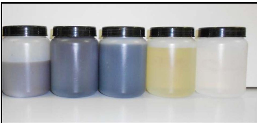
Figure 2: Photograph of the obtained samples (from left to right: raw OMW, after coagulation, UF permeate, NF permeate, RO permeate)
