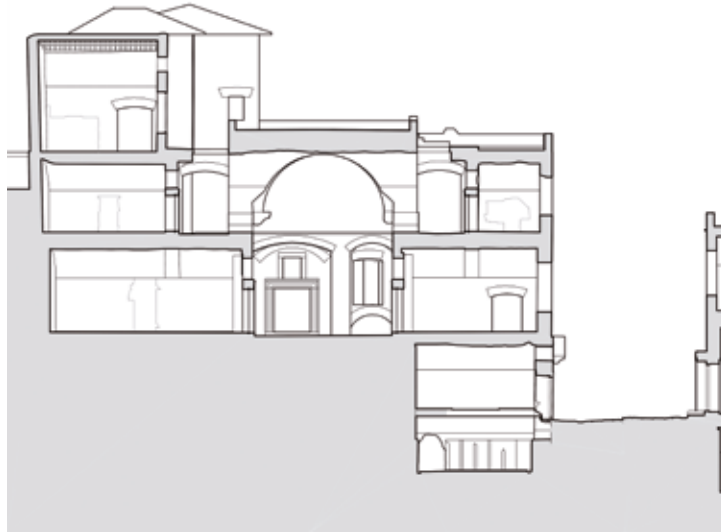
Fig. 1. The Great room, in the centre, which divides the Northern building, on the left, from the Southern one, on the right; note the lower level of via Biberatica respect the Hall.
