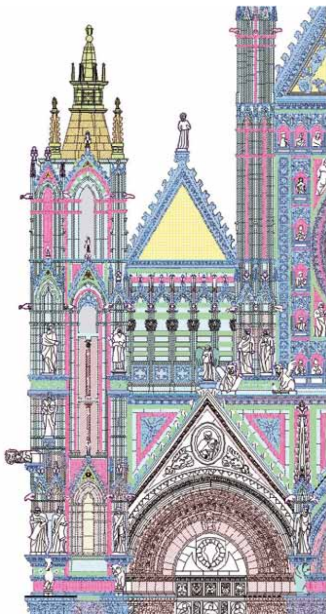
Fig. 2. Detailed project for restoration of Siena's Cathedral façade: mapping of single materials, different degradation states of conservation and different percentage of incidence of degradation for surface unit.
