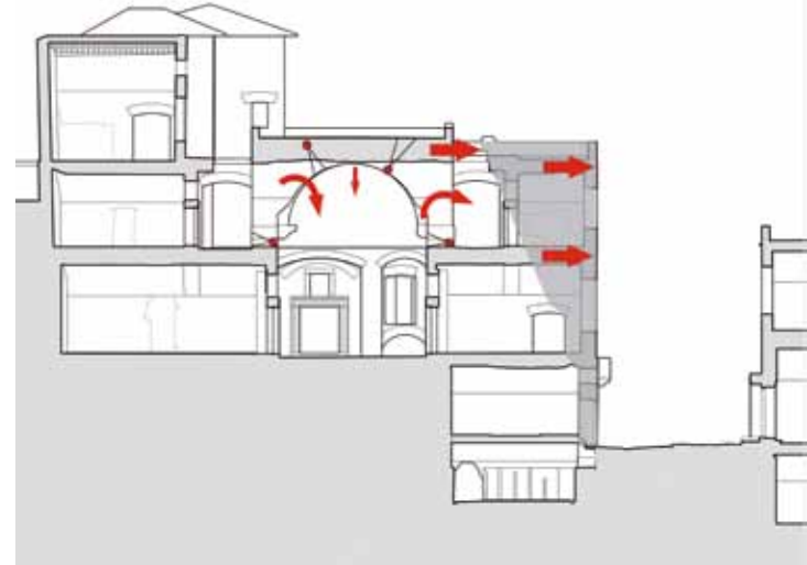
Fig. 2. The Southern building weak behaviour and the collapse mechanism in case of transversal seismic action.
