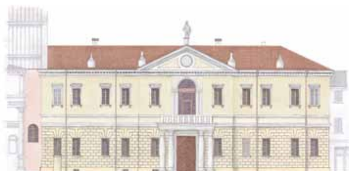
Fig. 5. Water colors painting to visualize the final result for restoration and coloring of a 18 th century façade of S Benedetto Po Monastery.
