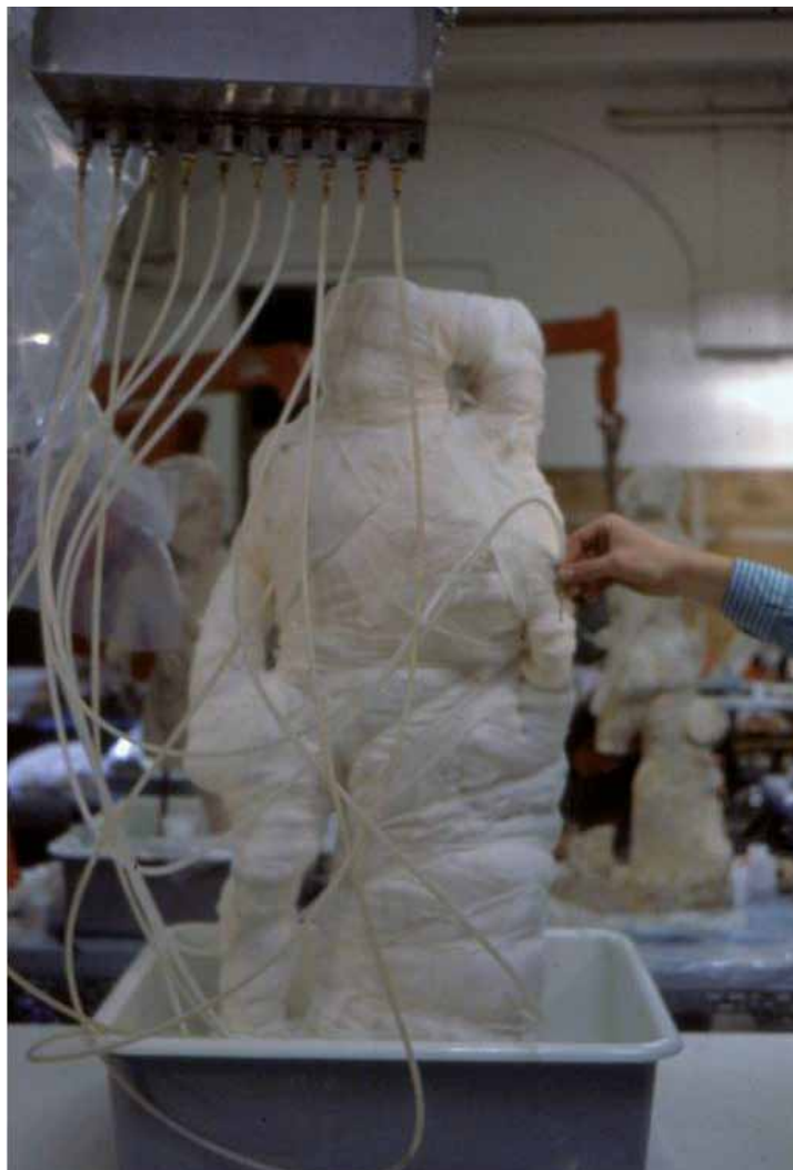
Fig. 11. Consolidation system by means of gradual imbibition.
