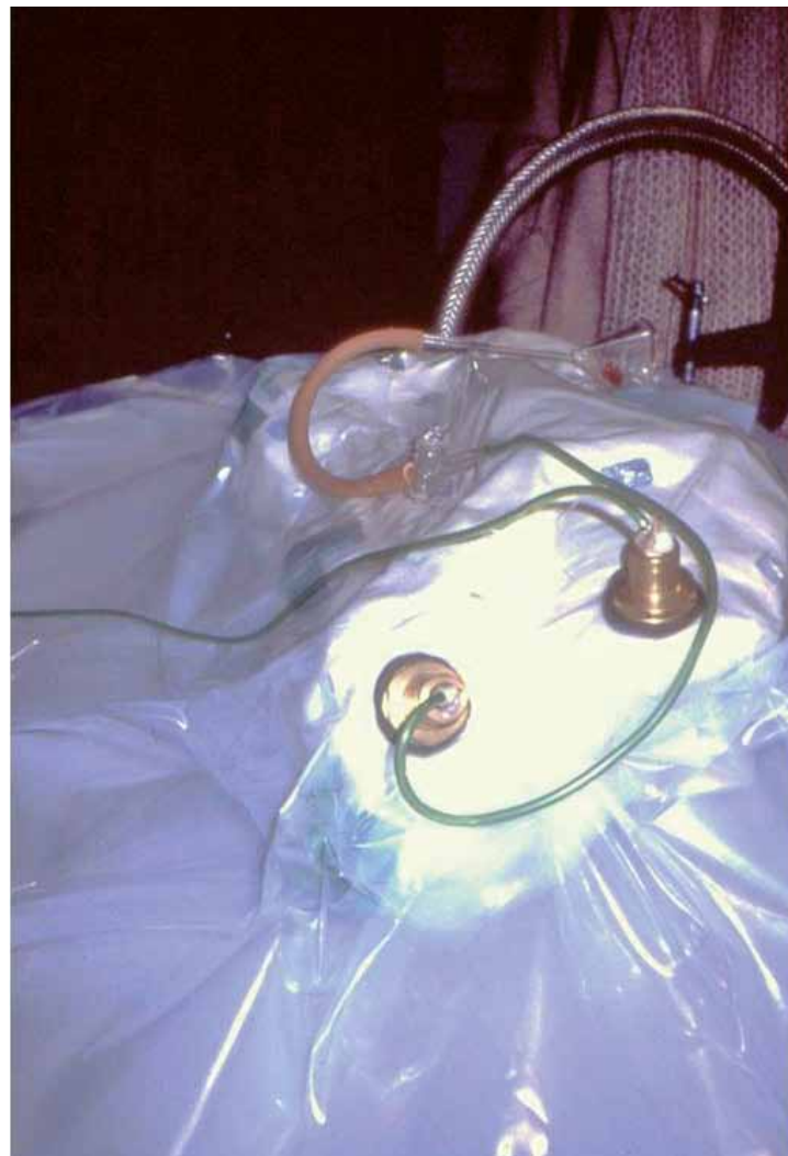
Fig. 12. Vacuum partial Consolidation System.
