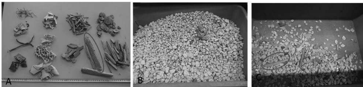
A: Example of input contaminants to the NIR sensor sorter, B: Accepted materials (NIR sensor sorting out put), C: Ejected materials (NIR sensor sorting out put)
