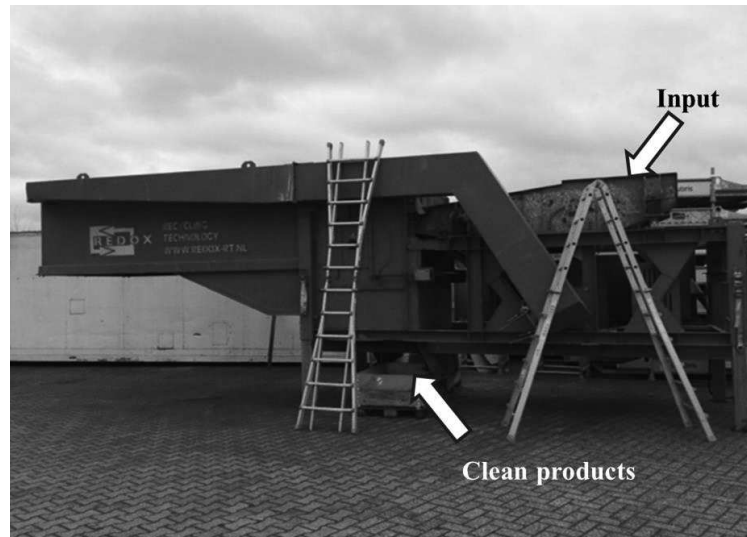
Figure 10: Wind sifting facility in REDOX.
