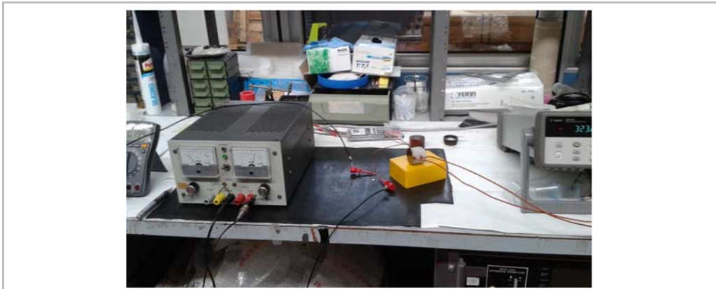
Fig. 1. Experimental set up for the measurements of the thermal conductivity.
