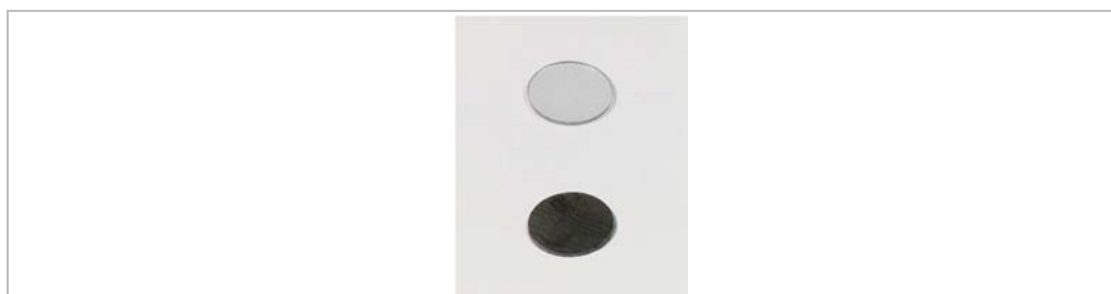
Figure 2: Comparison between a transparent and a “textured-black” diamond plate.
