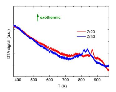
**Figure 2.** Differential thermal analysis (DTA) measurements on the two amorphous membranes conducted with a temperature rate of 4 K/min after subtraction of the background records with empty crucibles.
