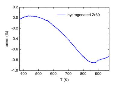
Figure 4. TGA scan of the hydrogenated Zr30 sample.
