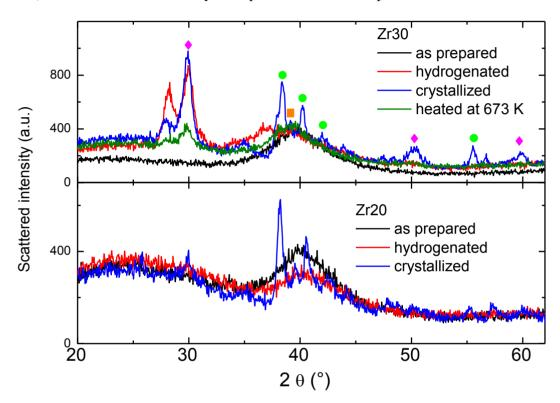
**Figure 1.** X-ray diffraction (XRD) spectra of all samples with attribution to crystalline phases (magenta diamonds: ZrO<sub>2</sub>; green solid circles: Ni<sub>10</sub>Zr<sub>7</sub>; orange squares: Ni<sub>48</sub>Zr<sub>52</sub>) [18–22].
