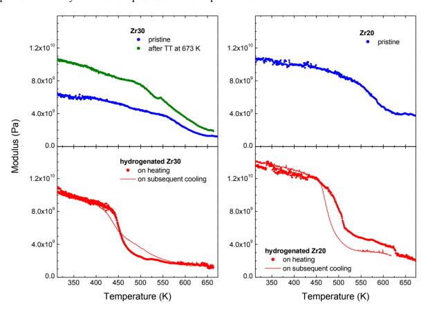
Figure 3. Dynamic Mechanical Analyzer (DMA) measurements of the membranes.
