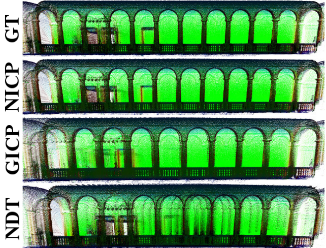
Fig. 1. Side views of the reconstruction of the ETH Hauptgebäude dataset. From top to bottom: ground-truth, NICP, GICP and NDT reconstruction. NICP was able to reconstruct consistently the scene while both NDT and GICP generated a shortened corridor ( count the arcs ).
