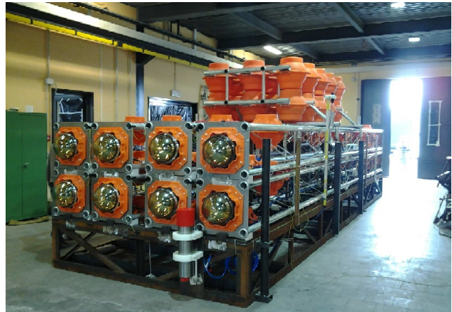
Fig. 5 The NEMO Phase-2 tower in its compact configuration during the integration phase.
