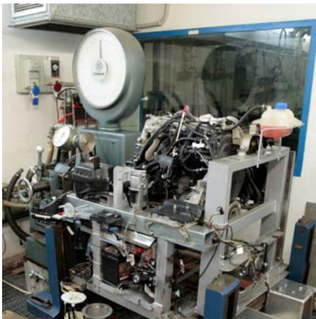
Figure 1. The FIAT 1.9 JTD Multijet engine used for the tests campaign.
