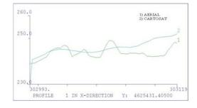
Fig. 12: profiles through a Cartosat-1 DSM and the reference DSM from aerial images an urban area
