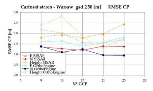
Figure 6. RMSE at check points trend for Warsaw image (North, East, Height components)
