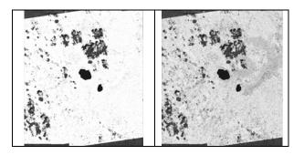
Fig. 9: matched image points (left) and quality image (grey values correspond to correlation coefficient) of Castelgandolfo
