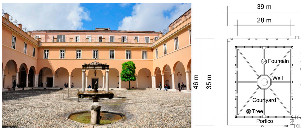
Figure 1. Dimensions and present configuration of the Cloister of the Faculty of Engineering of the “Sapienza” University.
