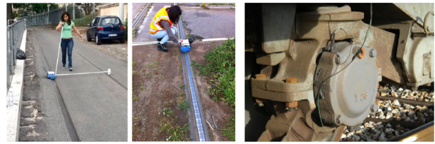
Fig. 6 Instruments for measuring the longitudinal profile of the rail (rail measurement)
