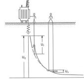
Figure 1. The ground potential rise (GPR)  $U_G$ , the touch voltage  $U_t$  and the step voltage  $U_s$ .
