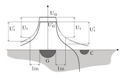
Figure 6. Potential behaviors of a hemispherical electrode with a single C current electrode at remote point (dashed line) and at short distance (continuous line).
