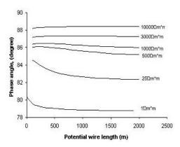
Figure 5. Phase angle  $\phi_{CE}$  in dependence of the potential wire lengths and the soil resistivity for impedance of the coupling effect
