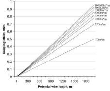
Figure 4. Curves of coupling effect Z<sub>CE</sub> (as impedance amplitude) versus potential wire length up to 2,000 m and different soil resistivity
