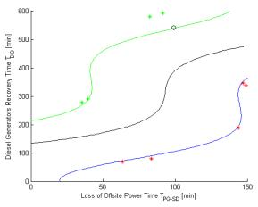
Figure 3: Initial limit surface after a very small training set (failure red, success green) [4].
