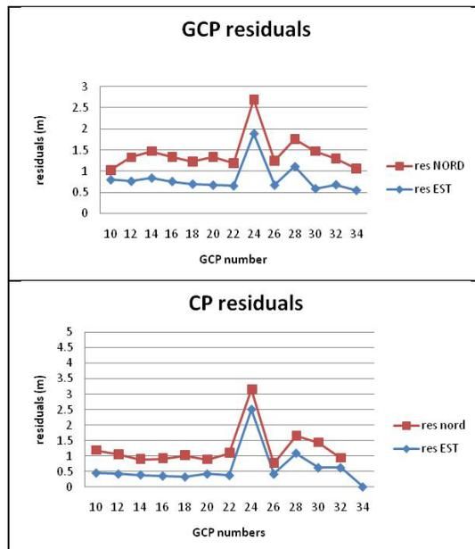
**Fig. 5.** Graphs of precision and accuracy obtained with third order polynomial function.
