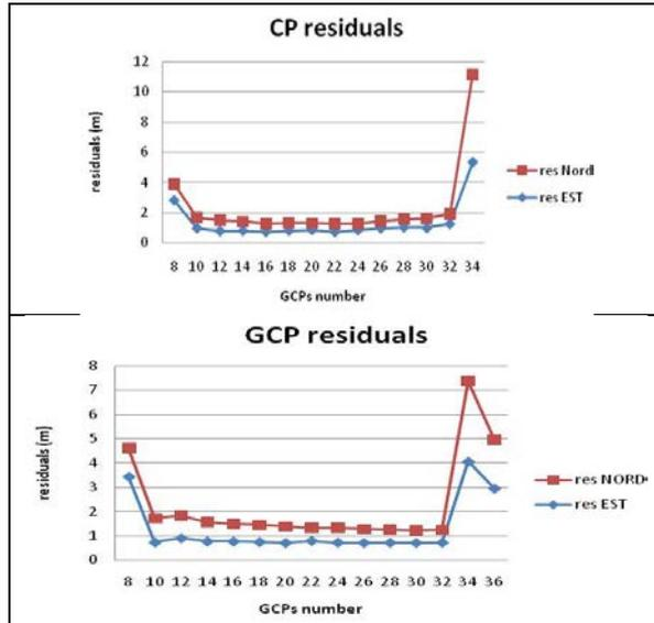
**Fig. 4.** Graphs of precision and accuracy obtained with second order polynomial function second test.
