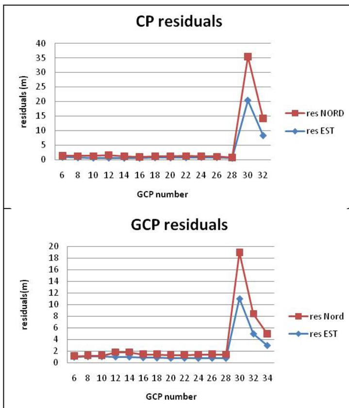
Fig. 3. Graphs of precision and accuracy obtained with second order polynomial function.
