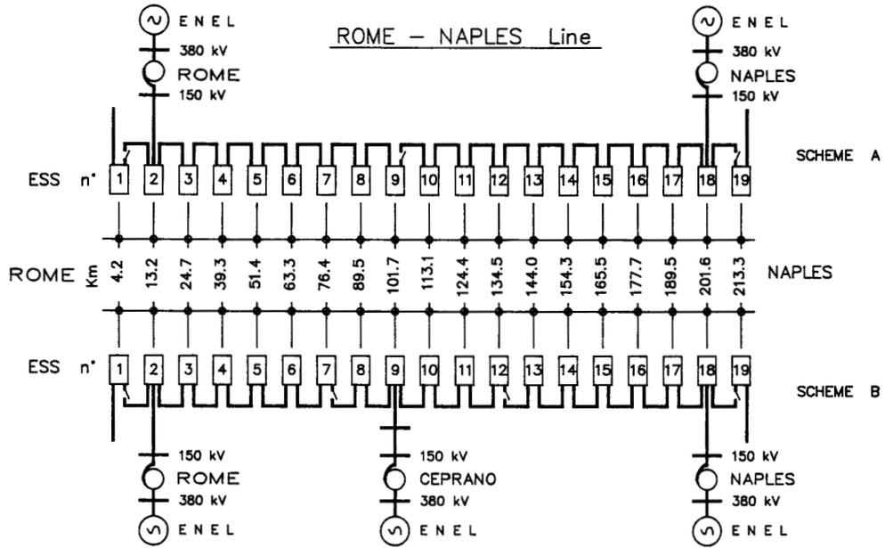
Fig.2-Traction Substation location along the railway line and HV supply line schemes.
