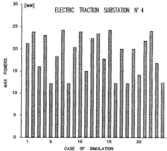
Fig.3-Maximum instantaneous powers for different departure time delays.
