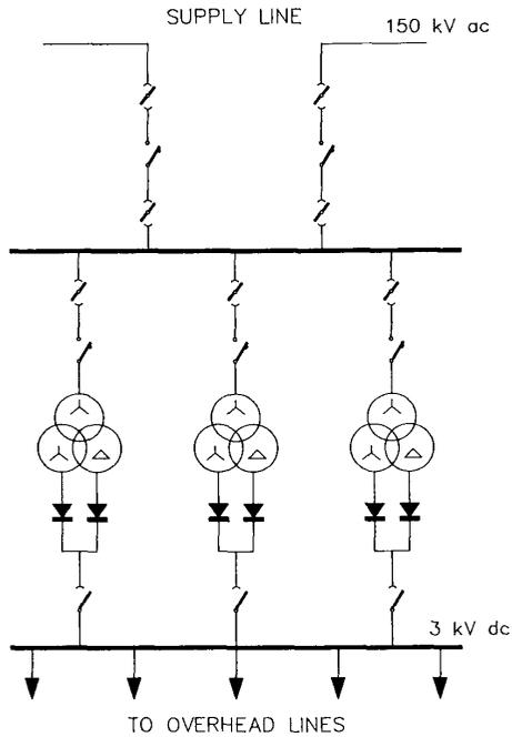
Fig.1-Electric Traction Substation scheme.
