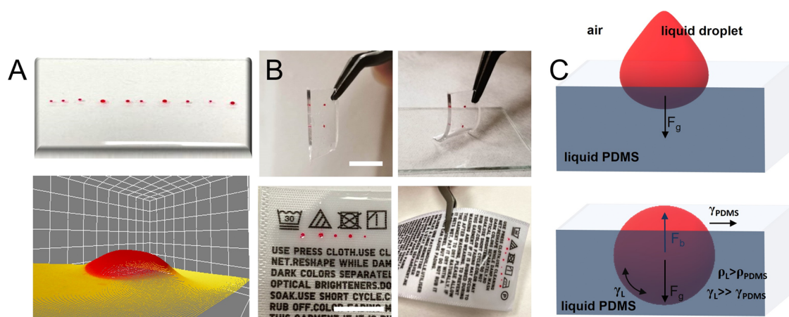
Figure 1. (A) Photograph of the smart WGM lasing device obtained via the spontaneous self-formation of 3D active microdroplets of a gain solution in a liquid elastomeric matrix. Such a polymeric device is realized by a random sequence of microdroplets characterized by different sizes and different compositions of dielectric particles included into the gain medium and compatible with a barcode reading. Below, the 3D reconstruction of the optical images of a droplet section outside the elastomeric matrix before encapsulation. (B) Images of the WGM device realized on a polymeric matrix (top) and on a clothes' tag (bottom). The pictures show the free-standing structure of both labels which can be realized on multiple substrates, detachable and reusable. Scale bars correspond to 1 cm. (C) Spontaneous, single-step droplet formation due to a viscoelastic dewetting between two immiscible liquid phases: a gain solution of dye-doped diethylene glycol [rhodamine B (RhB) in DEG] and a liquid slab of polydimethylsiloxane (PDMS). The condition for a spherical shape of the lasing droplet is guaranteed by the density difference ( \rho_L > \rho_{PDMS} ) and the interplay of surface tensions ( \gamma_L \gg \gamma_{PDMS} ).
