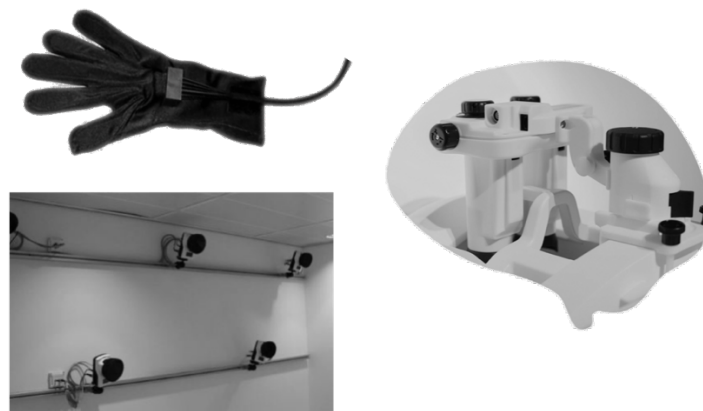
Figure 6.1. Components of MOTUM system: the amagnetic glove, the MRI-compatible cameras, and the VR glasses.
