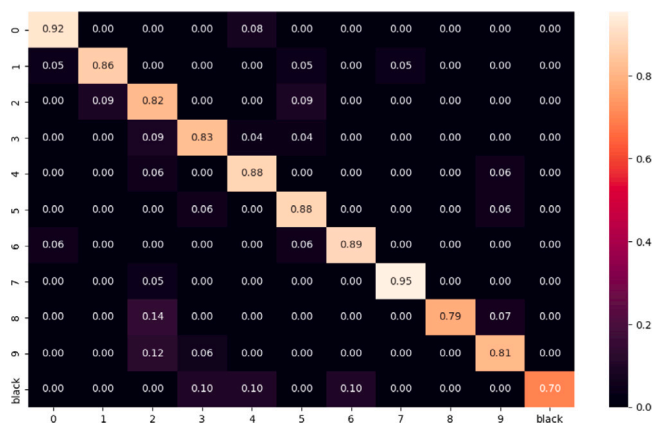
Fig. C.20. Confusion matrix resulting from RieManiSpectraNet+ architecture. The decoding performance for each class has been computed. When compared to Fig. 10(a), it is evident that all previous difficulties in distinguishing the classes have been resolved, thereby confirming that the RieManiSpectraNet+ architecture has achieved better integration of both spatio-temporal and spectral features.
