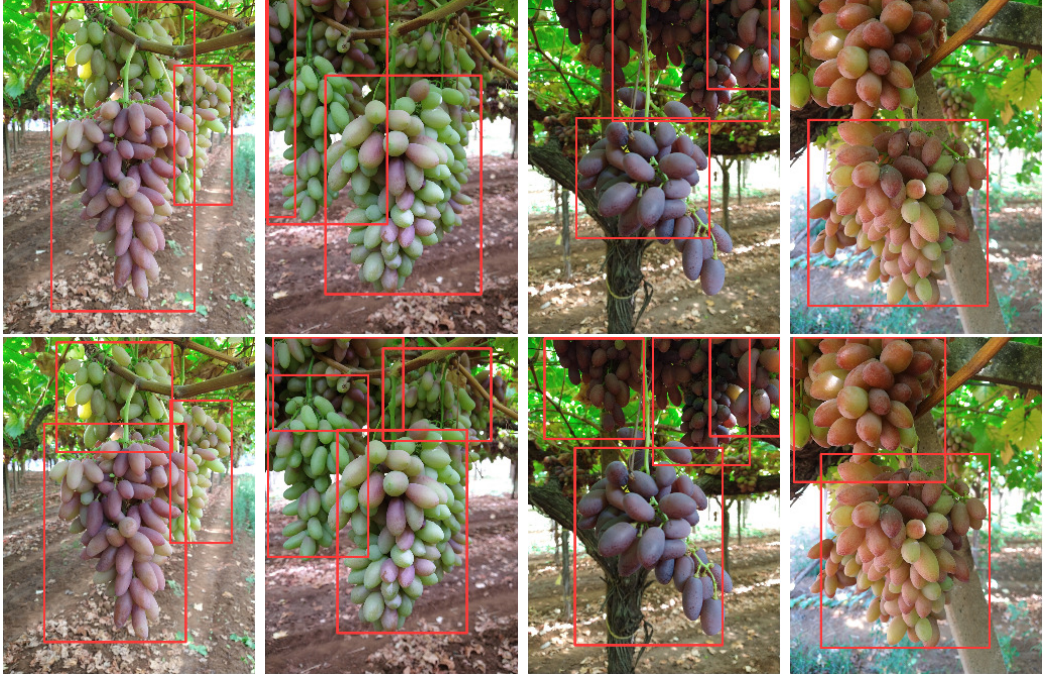
Figure 3.12. Qualitative comparison of object detection performance before and after domain adaptation. The top row illustrates the predictions generated by the baseline source detector (SDet), which struggles with missed instances and loosely fitted bounding boxes. The bottom row displays the predictions from the target detector (TDet) trained with surrogate supervision, demonstrating tighter localizations and significantly higher recall, particularly in dense and occluded canopy clusters.
