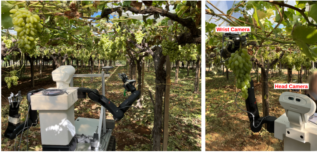
Figure 6.1. The robotic harvesting platform deployed in the experimental vineyard. Accurate quality assessment relies on the wrist-mounted and head-mounted RGB sensors to perform real-time Soluble Solid Content (SSC) estimation, simulating the visual checks performed by human workers.
