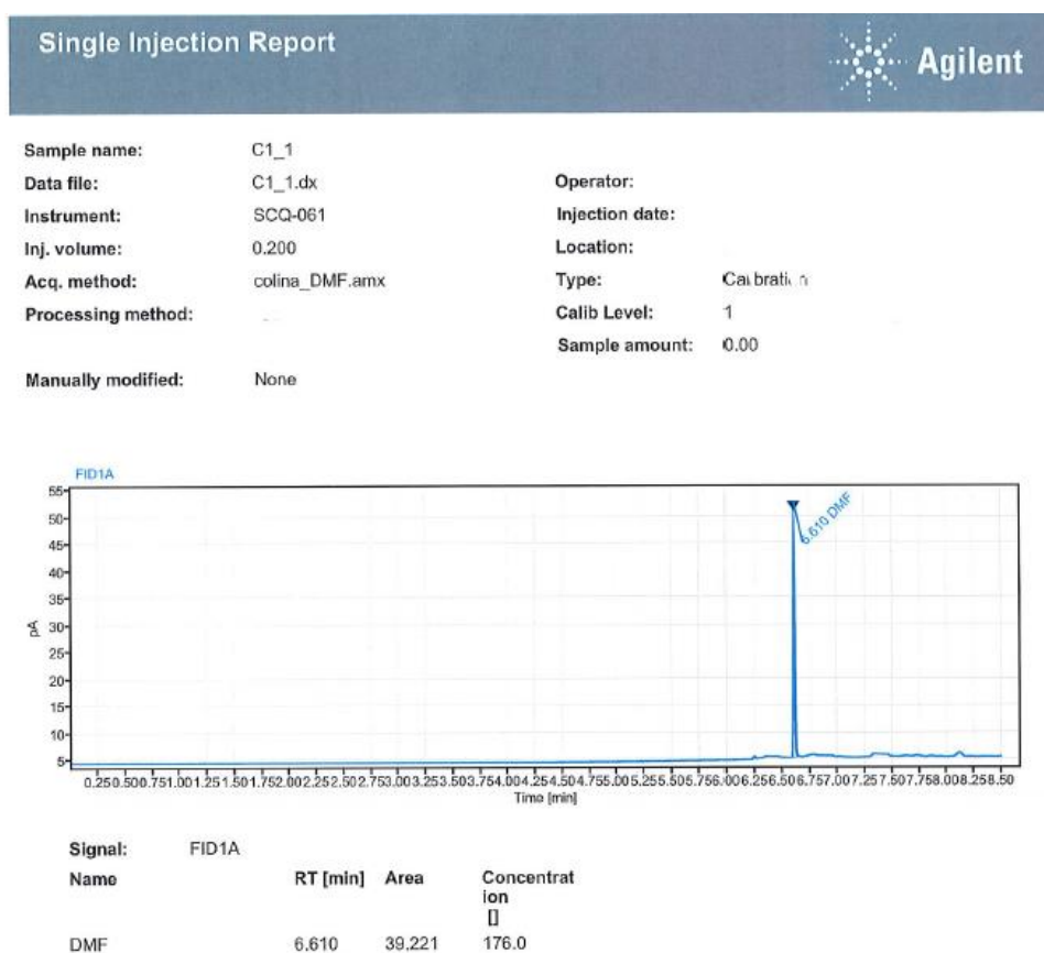
Figure 25. Linearity test, injection of mixture C1. First replicate to be tested.
