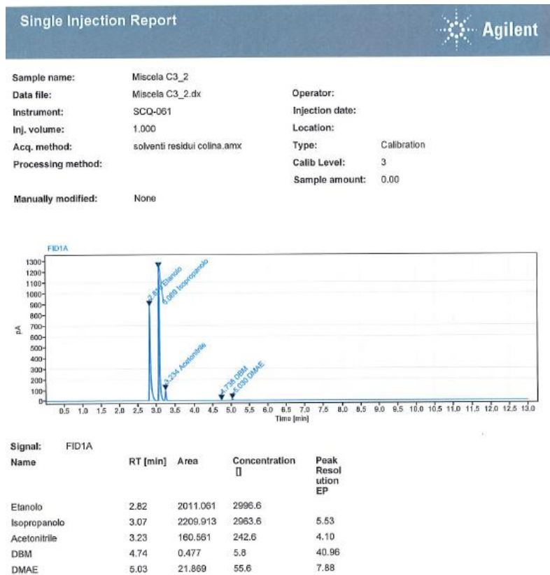
Figure 18: Linearity test, Mixture C3 injection. Third concentration to be tested
