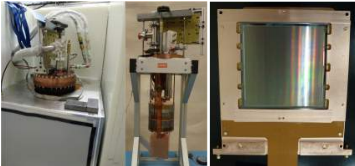
Figure 13: From left to right: Photographs of the DAMIC detector at SNOLAB showing the sealed copper cryostat inside its radiation shield, with electronics and service lines connected to the feedthrough flange, of the cryostat insert showing the Kapton flex cables running from the CCD box to the vacuum interface board along the channel in the internal lead shield, and of the DAMIC CCD module housing a 4k x 4k pixel CCD. Figures from Refs. [67, 68].
