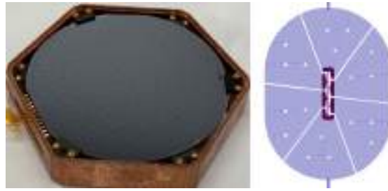
Figure 11: Left: A picture of the CPD installed in a copper housing. The instrumented side is shown facing up. Right: The design of the QETs used for the detector (blue: Al fins; purple: W TES). Figure and caption from Ref. [55] 4 .
