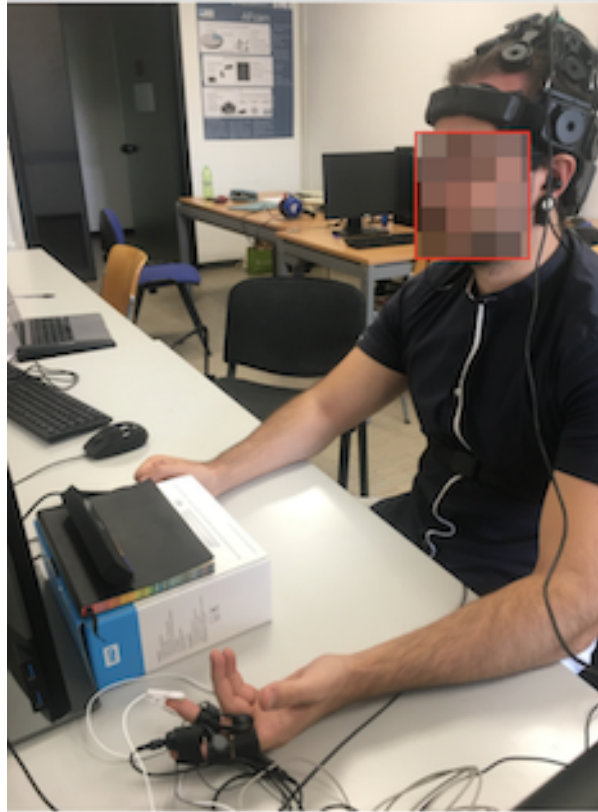
Figure 3.12: The set up used for the experiment. On the left hand of the subject is possible to see the BVP and GSR sensors of the Procomp device. On the box in front of the subject is possible to see the Tobii Pro X2 Compact eye-tracker and on the head of the subjects the DSI 24 headset is shown.
