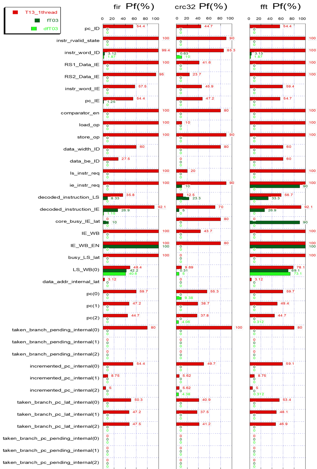
Figure 4. Fault-injection results with a Time Frame Spanning approach for the T03, ft03, and dft03 cores, running the FFT, CRC32, and FIR benchmarks. Target registers on the vertical axis and failure probability (%) on the horizontal axis.
