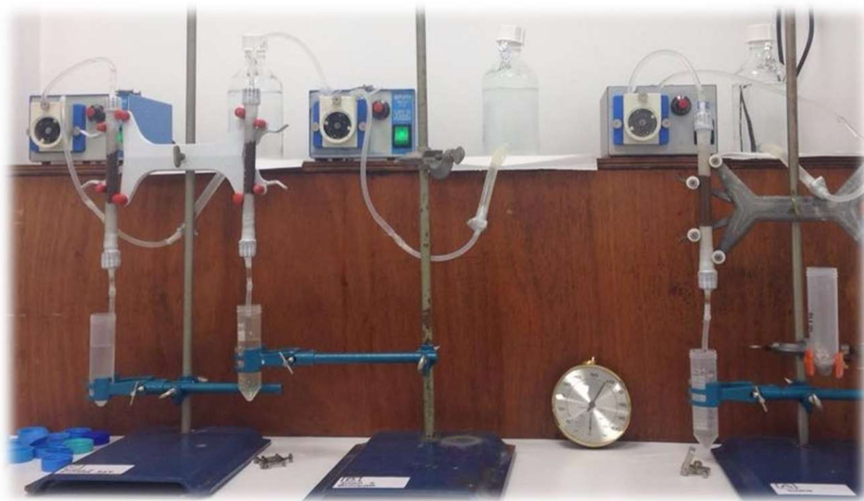
Figure 3.61 – Photographic documentation of the filled columns, connected to the peristaltic pumps.
