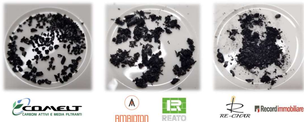
Figure 2.3 – Carbon-based sorbent investigated for physical-chemical characterization.
