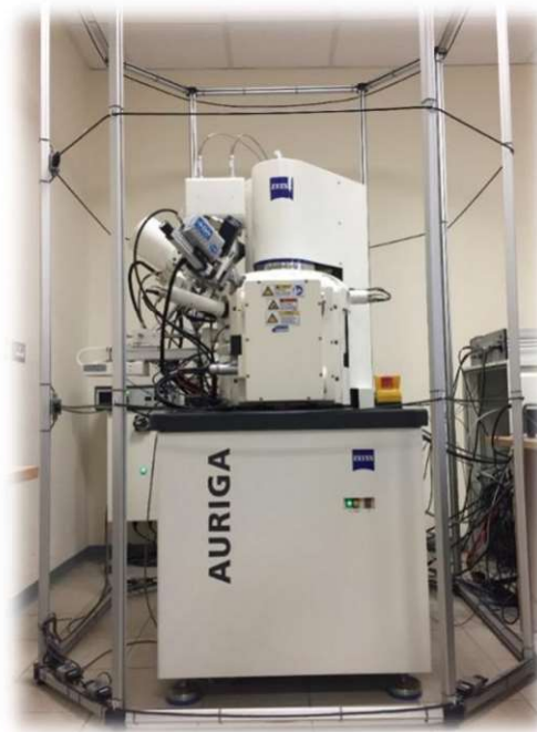
Figure 2.5 – HR FESEM Zeiss Auriga at the CNIS (Research Center for Nanotechnologies applied to Engineering).
