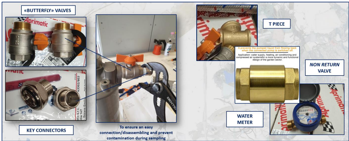
Figure 17. Filtration System components.
