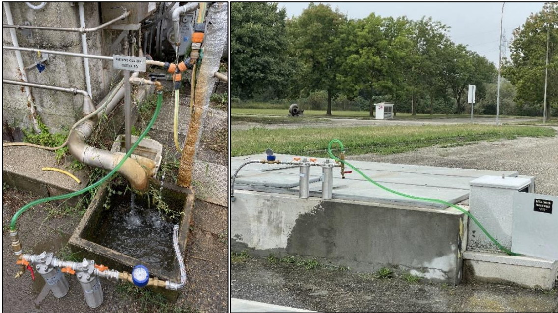
Figure 23. Sampling setup for the filtration system in DWTP #3: surface water (left) and drinking water (right).
