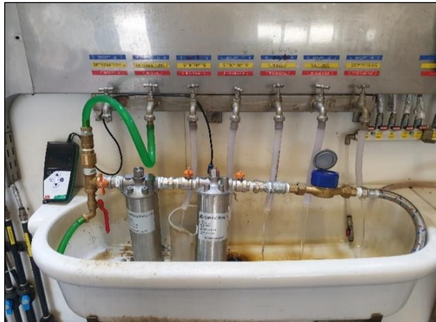
Figure 22. Sampling setup for the filtration system in DWTP #2: surface water (up) and drinking water (down).
