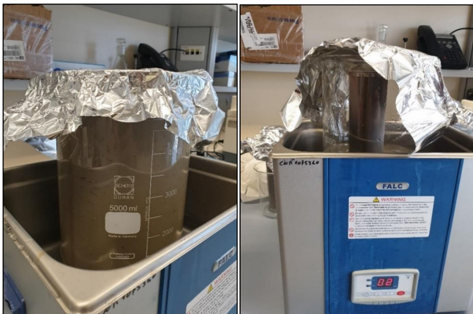
Figure 24. Resuspension of particles for a surface water sample (left) and a drinking water sample (right).
