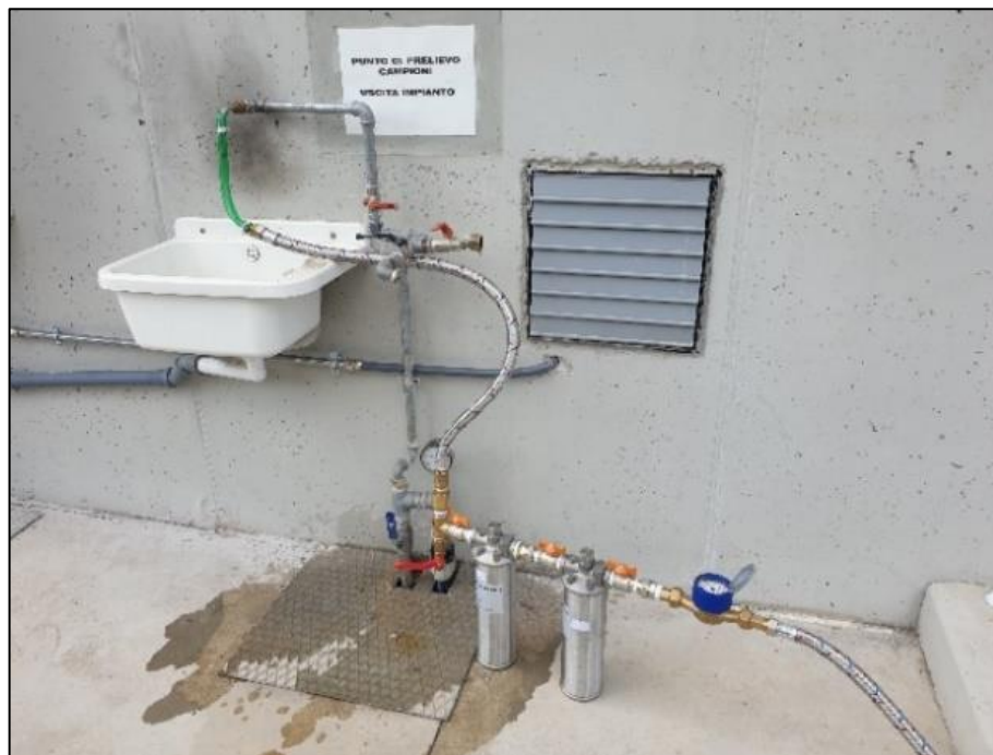
Figure 20. Sampling setup for the filtration system in DWTP #1: surface water (up) and drinking water (down).
