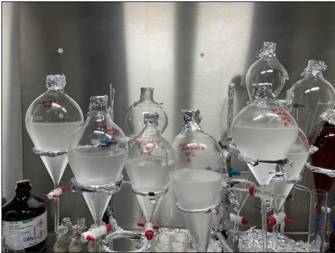
Figure 26. Digestion/Extraction for Drinking Water DWTP #3 Samples.
