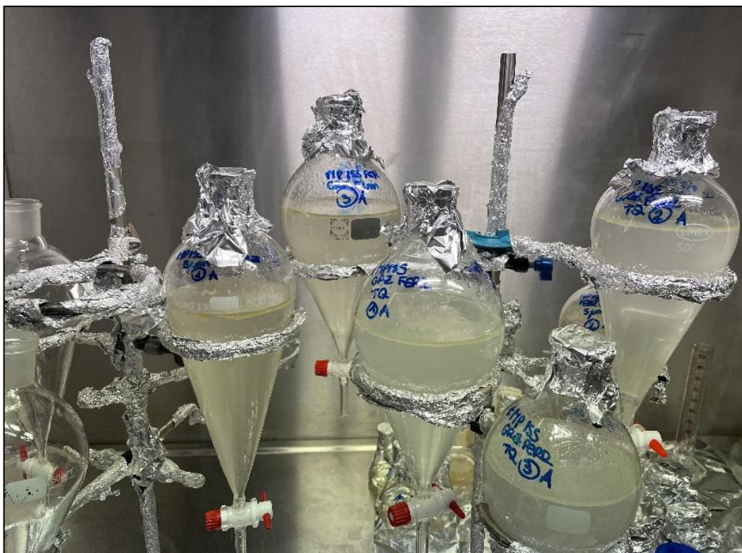
Figure 25. Microplastics digestion/extraction for surface water DWTP #3 samples
