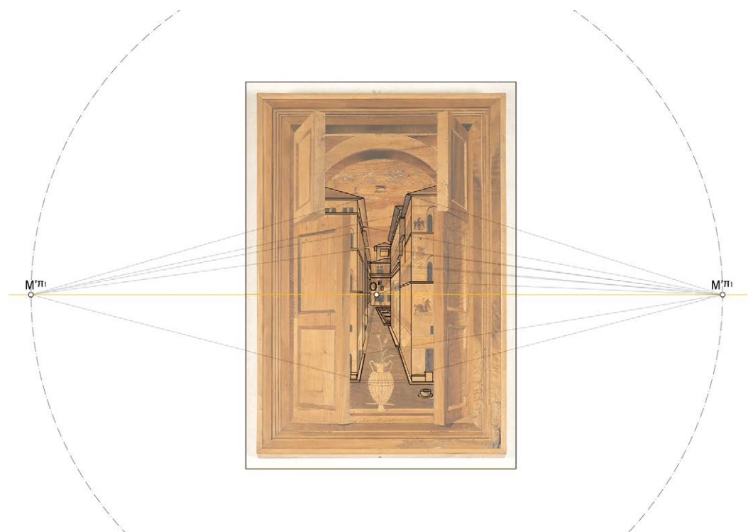
Fig. 5. Research of fundamental perspective entities. The vanishing point and the horizon line identified by leading perpendicular lines to the picture plane into convergence; the projection center in space was determined by considering lines at 45^\circ , defining the circle of distance.
