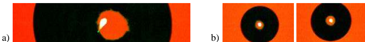
Fig. 7 Superimposition of plasma (yellow), bubble at maximum radius (black disk) and maximum radius of the first rebound (small red disk). (a) E_L = 26 \text{ mJ} , \gamma \sim 53^\circ and R_{\max} = 1970 \mu\text{m} . (b) E_L = 9.5 \text{ mJ} and \gamma \sim 12^\circ and R_{\max} \approx 550 \mu\text{m} .
