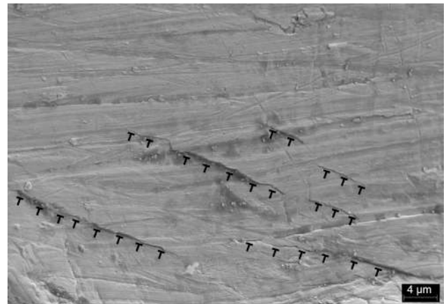
Fig. 17. SEM image of micro-cracks propagation along several dislocation planes aligned with the maximum normal strain plane ( \bar{\sigma}_{max} = 47.5\%S_u ).
